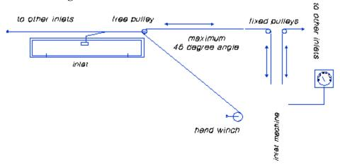
Figure 2. Hand Winch Installation to Reduce Inlet Speed.
