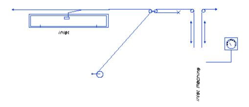
Figure 4. Hand Winch Installation to Keep Inlet Speed the Same As Inlet Machine Speed.
