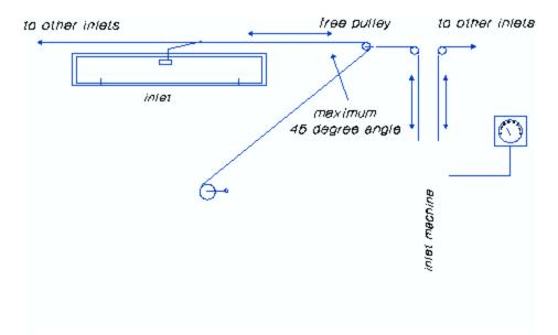
Figure 3. Hand Winch Installation to Increase Inlet Speed.
