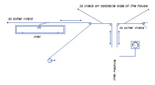
Figure 5. Hand Winch Installation to Increase Inlet Speed in Long Houses.
